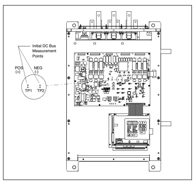
Figure 6.1 – DC Bus Voltage Terminals (414 Amp Drives)
